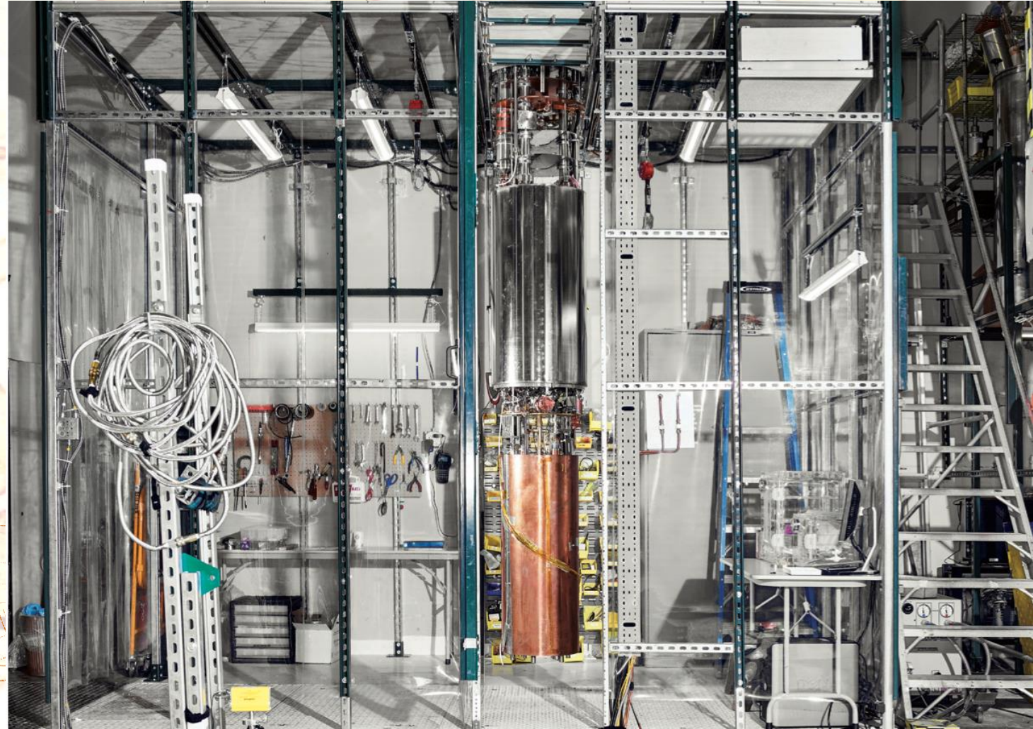
Axions (and Axion Like Particles) Cavity & multistrip SQUID amplifier @ sub K \rightarrow Sensitivity at quantum limit
