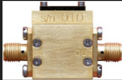
HEMT amplifier from Low Noise Factory
