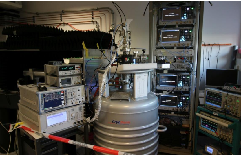
Test setup with 4 samplers and fake axion injection: Detection of 1.2 \times 10^{-22} W signal within few days
